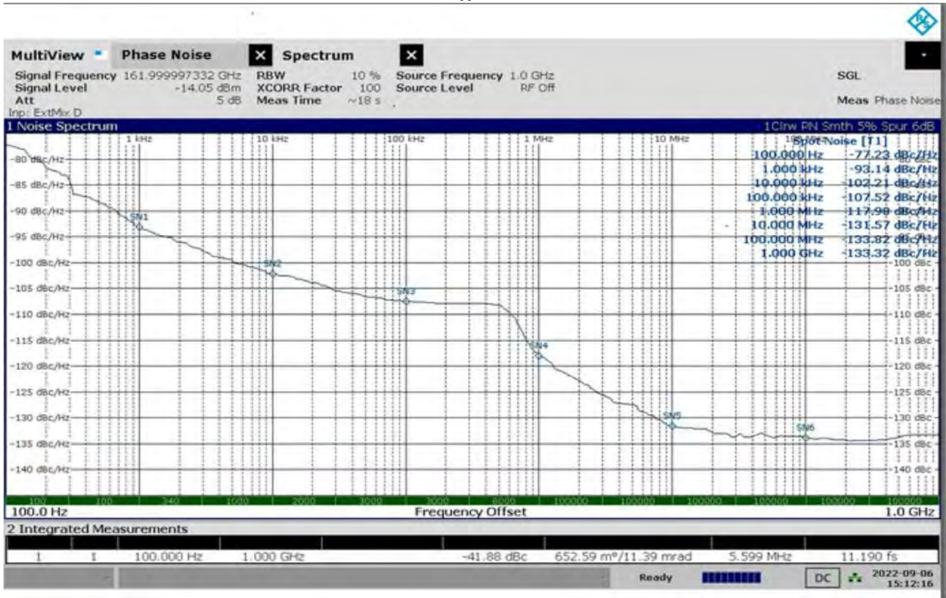
Figure 3: Measured Phase Noise of a PLL System at about 162 GHz using the R&S FSWP Signal Source Analyzer
